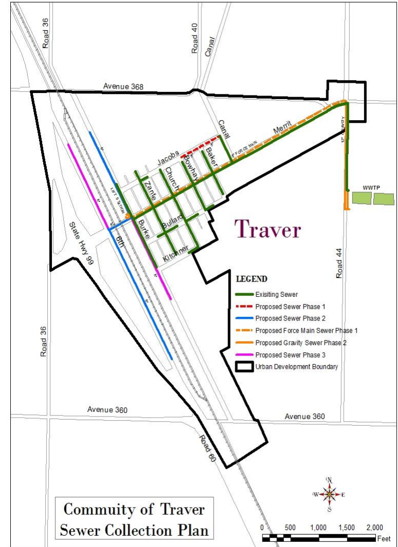
Figure 8 – Community of Traver Sewer Collection Plan
